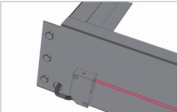
The Photo Sensor is installed to the front edges of the mobile units. Produces a highly sensitive infrared beam to monitor obstructions.
