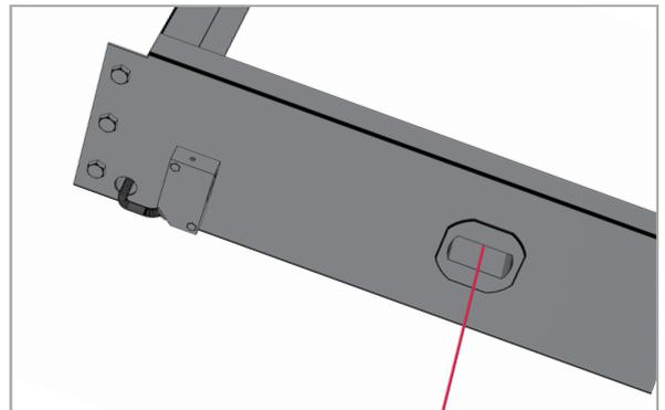
The Distance Sensor is installed to the front of the mobile unit. It stops movement of the carriages if an object or person enters the aisle.
