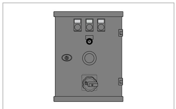
The Power Unit Connects to 240V power and converts output power to 24V DC. Can also be turned on using remote control.
