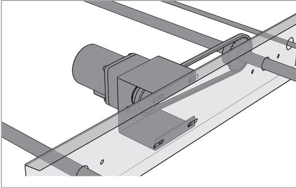
The 40W DC motor c/w 100:1 reduction gearbox provides plenty of torque to move up to 15T. This allows each unit to hold an incredible amount of weight, and have it shifted effortlessly on a low voltage system.
